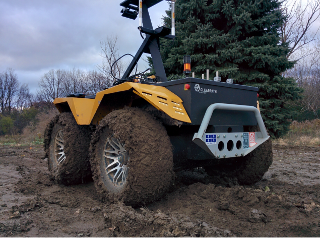
Fig. 3: This figure shows the 900kg Clearpath Grizzly on the muddy test track used for the experiments in the results section. The controller receives estimates of its pose and velocity from a vision system which relies solely on a stereo camera (c.f. [23]).
