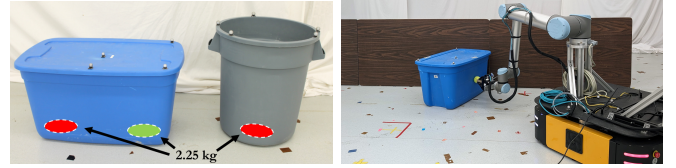
Figure 10: Left : The “Box” and “Barrel” sliders used for real-world experiments. Each is empty except for 2.25 kg weights located approximately at the colored circles. The red weights are always present, but we add or remove the green weight to vary the mass and pressure distribution of the box. When both weights are present, we refer to the slider as “Box2”; with a single weight it is called “Box1”. The Barrel has radius 20.5 cm, height 56 cm, and total mass 4.5 kg. The Box has width 65 cm, depth 33 cm, and height 43 cm; the total mass of Box1 is 4.8 kg and of Box2 is 7 kg. The friction coefficients with the ground were estimated to be approximately 0.3–0.4 on average for both objects. Right : The robot pushing the Box along the curved trajectory, shortly after the slider first makes contact with the “wall” (we use overturned tables).
