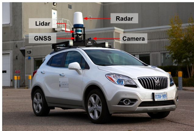
Fig. 1. Our data-taking platform, Boreas , which includes a Velodyne Alpha-Prime (128-beam) lidar, Navtech CIR204-H radar, FLIR Blackfly S monocular camera, and Applanix POSLV GNSS.
